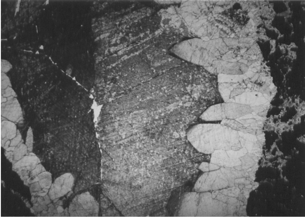
Figure 3. Two generations of fracture cement; field of view is 1.8cm
